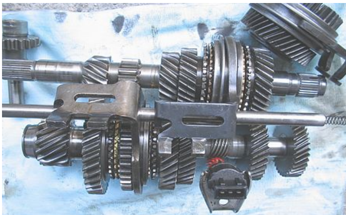
Figure 1.1: A five speed gearbox with gears connected to shafts
